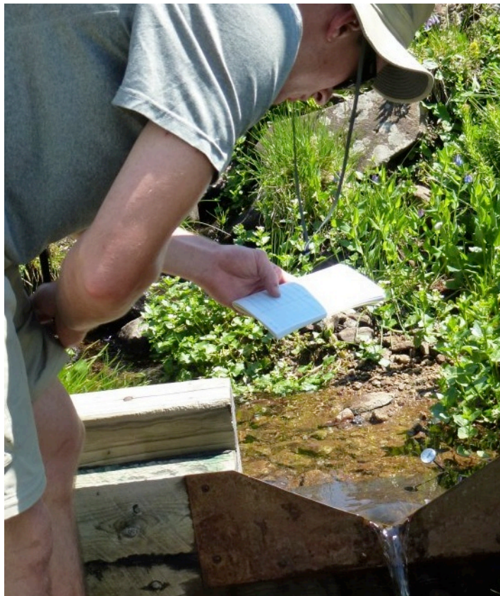
Figure 29. Measuring water temperature with the analog (“old”) thermometer at the Saddle weir (location 009).
