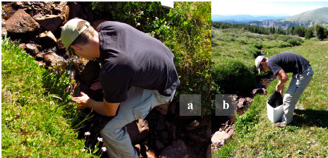
Figure 26a. Using a heavy duty trash bag to measure discharge in a stream channel in Saddle stream and b. consolidating collected discharge into a graduated bucket.
